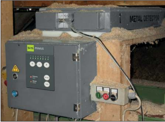
Installation example: Plate type detector ELS with control unit PRIMUS analysing wood off-cuts (old version)
